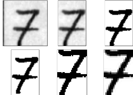
Figure 2: Preprocessing steps: Original, Horizontal Cropping, Binarization, Centralization, Symbol-Cropping, Resizing.
